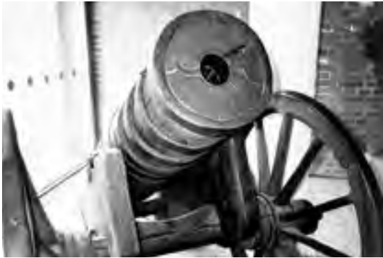
Fig. 4.54. Front view of a cannon from the German National Museum in Nuremberg. The wooden trunk surrounding the inner, metal, is bound on the outside with hoops for strength. Probably, field guns were lightened in this way. Photo of 2000.
