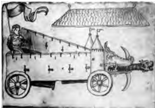
Fig. 4.13. The Iron Chariot is probably a large cannon on four wheels. The cart-carriage, apparently, is bound with riveted iron. A drawing from the “Treatise on Throwing Weapons,” 80s of the XV century [739], p. 55. Taken from [739], ill. 9.
